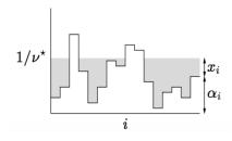
The height of patch *i* is given by  $\alpha_i$ . The region is flooded to a level  $1/\nu$ , using a total quantity of water equal to one. The height of the water (shown shaded) above each patch is the optimal value of  $x_i$ .
