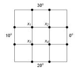
In this 2D example we wish to estimate the temperature at the nodes of the grid, based on four measurements at the boundary.
