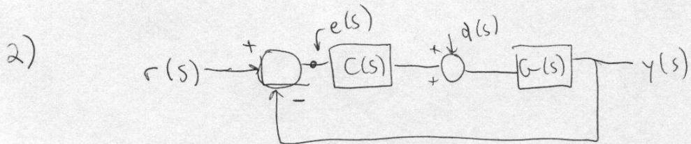
a) setting  $d(s) = 0$ , transfer function from  $r$  to  $y$  is
