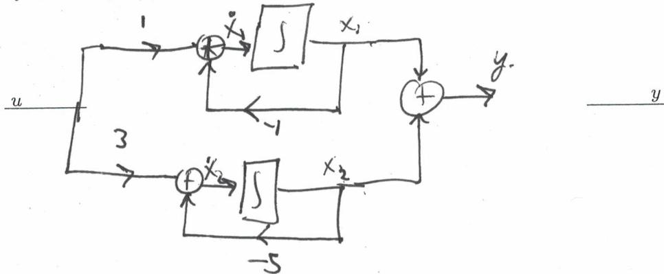
[2 pts] h) Draw a block diagram representation using integrator, scale, and sum components for the system in eqn. (2)
