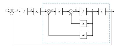
[3 pts] a. Write the state and output equations for the system, in terms of  $A, B, C, K, K_e$ .
