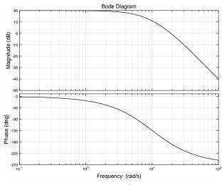
A lag controller  $D(s) = k \frac{s+\alpha}{s+\beta}$  is to be designed such that the unity gain feedback system with openloop transfer function D(s)G(s) has the same steady state error as with OLTF G(s)and has a nominal (asymptotic approximation) phase margin  $\phi_m = 55^\circ$  at  $\omega = 8$  rad  $s^{-1}$ . Note  $20 \log |G(j\omega = j8)| = 13$  dB.
