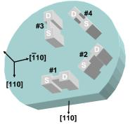
Perspective view of wafer with etched Si fins
