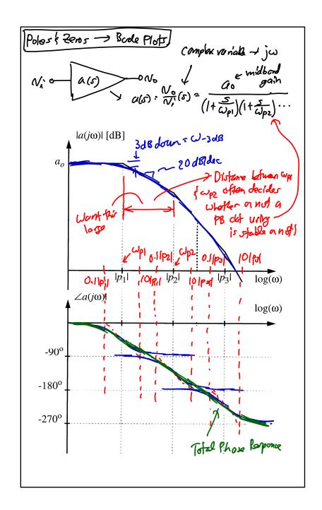
Free Response Recall that the transfer function of a general amplifier can be expressed as a function of frequency via: A(s) = AMF\_(s)FH(s) S=jw
