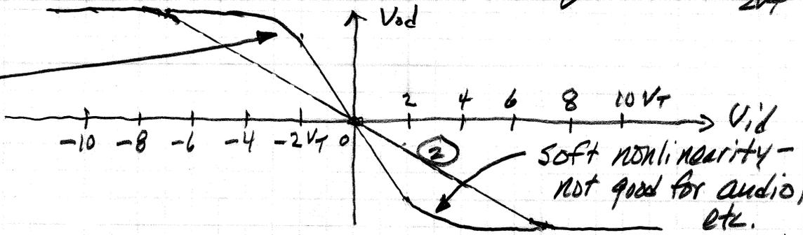
Only linear for  $-V_T < V_{id} < V_T$  (i.e.,  $|V_{id}| < 25\text{ mV}$ )
