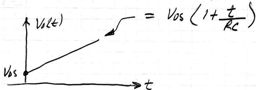
$V_o$  will rail at  $V_{DD}$  over time.
