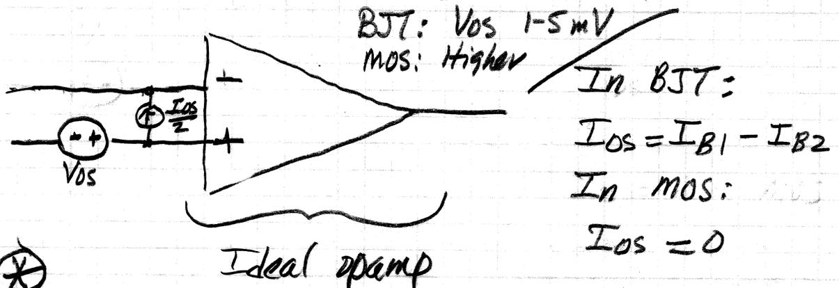
$V_{os}$  = Voltage needed in the configuration above to set  $V_o = 0$  (or  $V_{DD}/2$  as appropriate)
