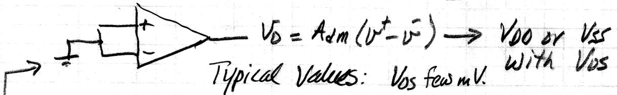
How to model - input-referred so as to be able to compare to the size of the input signal.
