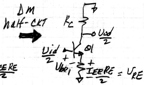
$$A_{dm} = \frac{-g_m R_C}{1 + g_m R_E} \approx -\frac{R_C}{R_E} \text{ for } g_m R_E \gg 1 \text{ (curve 2)}$$
