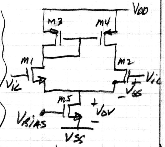
$$V_{ic(max)} = CMR^+ (m1 \text{ triode})$$
