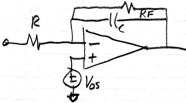
$$V_o = V_{os} \left( 1 + \frac{R_F}{R} \right)$$
