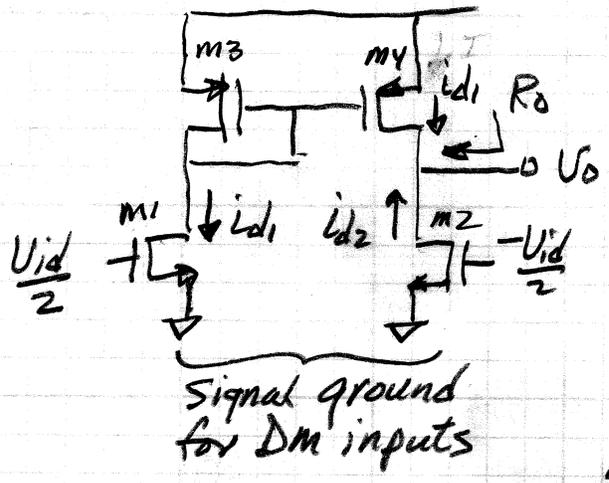
$$i_{d1} = g_{m1} \frac{V_{id}}{2} = g_m \frac{V_{id}}{2}$$
