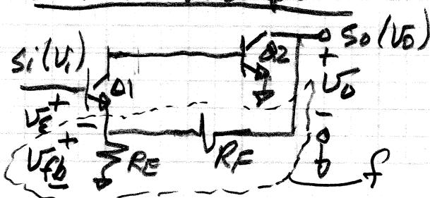
Series-Shunt: i.e., Voltage-Voltage
