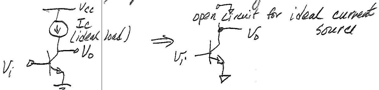
Quick S.S. analysis:  $A_v = \frac{V_o}{V_i} = -\left(\frac{g_m r_o}{1 + g_m r_o}\right)$
