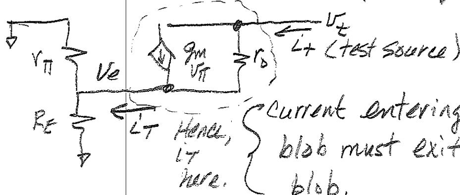
$$\therefore \text{by inspection, } V_E = \frac{i_T}{(g_\pi + g_E)}$$
