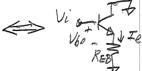
$$KCL: V_i = V_{be} + I_b R_B \quad KCL: V_i = V_{be} + I_e R_{EB}$$
