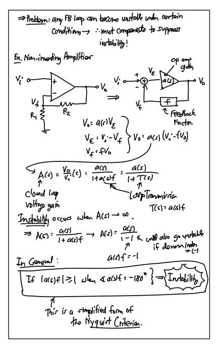
Stability of F13 Ckt. Using a single Pole Op Amp
