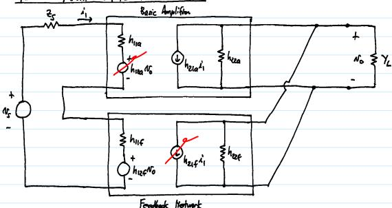
In gonal, transista amplifies & FB notworks are uni-directional -> they have large gains in the forward direction, but very small gains in the revowe:
