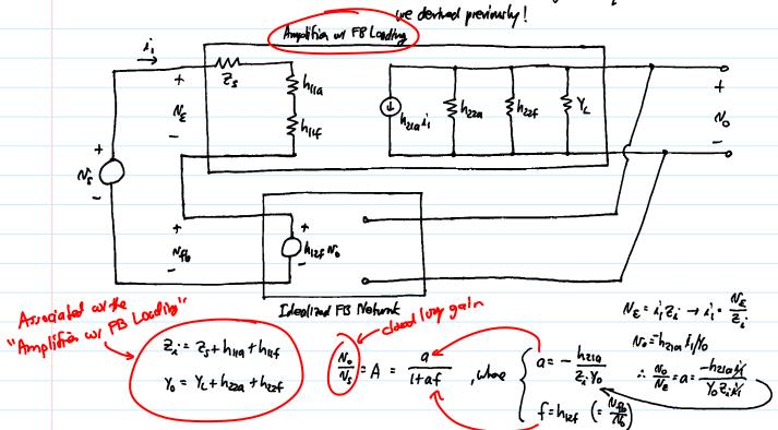
Thus, the kay to inspection analysis of FB chts: You FB impedames to load the basic amplifier, then use our "inspection" formules.
