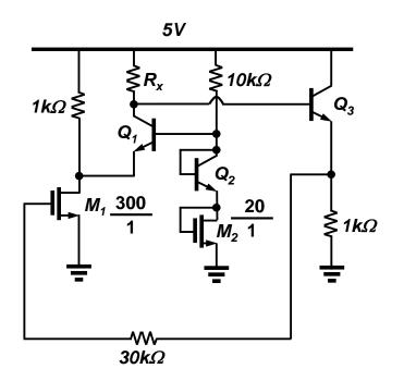
5. Consider a bias circuit shown below. Calculate the output voltage  $V_{out}$  and output current  $I_{out}$ . Assume  $V_{BE(on)}=0.7$ V and  $V_{CE(sat)}=0.2$ V.
