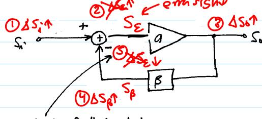
where  $S$  could be a current, voltage, displacement, etc., ...
