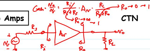
→ ideal when  $\frac{V_o}{V_+} = A_v$ ; i.e., when source and load R's do not influence the gain of the amplifier.
