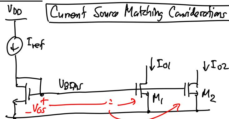
$$\therefore \frac{\Delta I_D}{I_D} = \frac{\Delta(w/l)}{(w/l)} - \frac{\Delta V_F}{(V_{DD}/2)}$$
