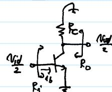
$$\text{By inspection: } \frac{N_{id}/2}{i_b} = \frac{N_{id}}{i_b} = A_{dm} = -g_m R_c$$
