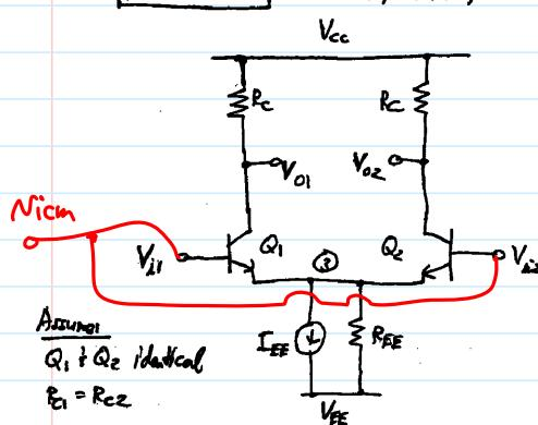
Purpose: Amplify the difference between two signals regardless of their common-mode DC values (or their common-mode values in general)
