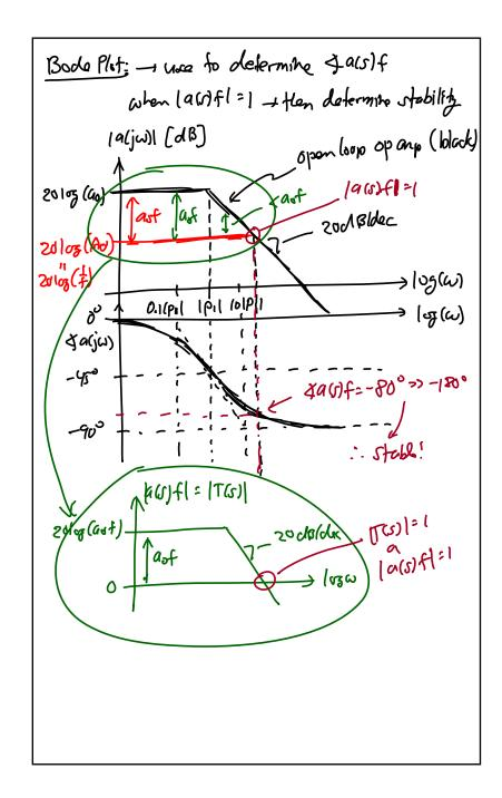
Remarker. 1) Fu the case of a single-pole op amp, FB can Novon reach \$ a(0) f = - 180 ° (90° is the limit) 2) Thur, an op amp FB c. t. w/ f: const. and Using a style pool op amp is always stable! But add a few non-dominant piles -+ thon instability is possible! sphoe now, & acosf can reach -170°s Can best visu lize this via a Bade plot.
