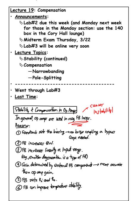
> Problems any FB log can become unstable undar certain conditions Sneed to componente the instabilities Ex. Non-Inverting Amplifies gaih Treedbood  $\frac{V_0(s)}{V_1(s)} = \frac{a(s)}{1+a(s)f} = \frac{a(s)}{1+\tau(s)}$ T(s)= a(s)f Closed Loop Loop Transmission Voltago Gain Instability occurs when A(s) -+ 0. = A(s): alstf: -1 Unstall when denominant = (-)
