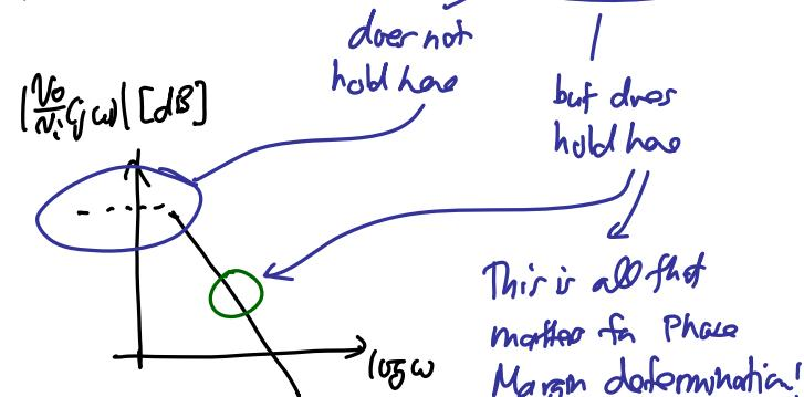
$$\left| \frac{V_o}{V_i(j\omega)} \right| = \frac{G_{m1}}{WC_c} \Rightarrow \text{this should equal } A_o \text{ @ the freq. } \omega \text{ corresponding to the target phase margin}$$
