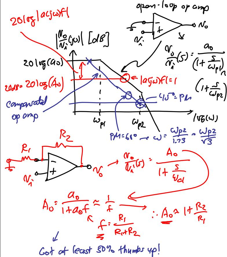
② Case 2: Two-Stage Amplifiers, Shunt  $C_c$  Compensation
