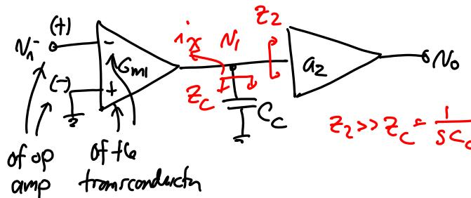
$$\left. \begin{aligned} N_1 &= -\frac{G_{m1} N_i}{sC_c} \\ N_0 &= a_2 N_1 \end{aligned} \right\} N_0 = -\frac{G_{m1} a_2}{sC_c} N_i$$
