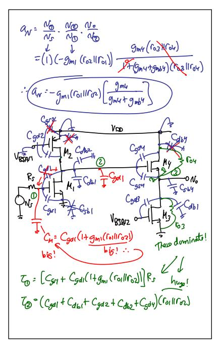
$T_{3} = \left(C_{db^{3}} + C_{gd^{3}} + C_{sb^{4}}\right) \left[\frac{1}{9m^{4} + 9mb^{4}}\right]$  $T_{gs4} = C_{gs4} \left( \frac{(r_{01}|1|r_{02}) + (r_{03}|1|r_{04})}{p_{f}(g_{my} + g_{mb} +)(r_{03}|1|r_{04})} \right) \times$ from impochion formula 2 but - there's a 2000, 3my + 5mby tor, in Mas  $\omega$ WH: To+ To+ To+ Tory
