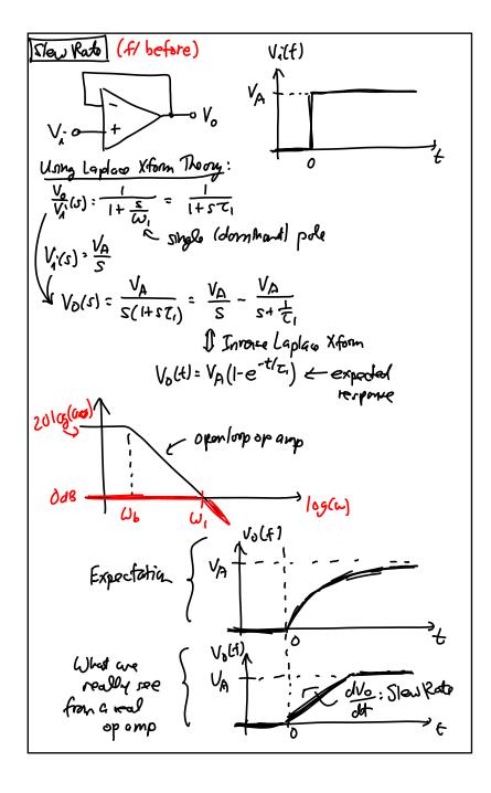
Reasons 1st on 2nd stage of op amp cannot source encych current to mimic the slope (a speed) of a fast vising input signal LXN C+Q [ [(21,) dt -Q-My 27 ZI, J.R.: Stew Rate dt mirro If opply a very fast (i.e., high fraquency), large amplitude shuroidi teoretically expected arthret V.(K) Slane: SR
