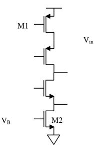
Given the bias voltages above, what are the bias voltages at the sources of the cascode transistors, and what is the output swing? Assume that  $|V_{tp}|=V_{tn}=0.5V$ , and that M1 and M1C have the same W/L, and that M2 and M2C have the same W/L.
