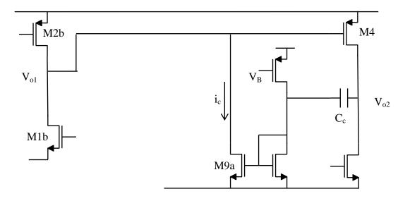
Now consider this circuit. What is the small-signal current  $i_c$  as a function of  $v_{o1}$ ? Does this circuit provide pole-splitting? Does this circuit remove the RHP zero?
