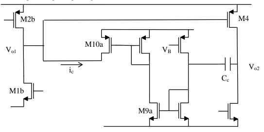
6) [28] In the two-stage op-amp below, assuming  $I_{ref}=10uA$  and  $(W/L)_6=(10u/1u)$ , design the amplifier so that the tail current is 20uA, the second stage current is 100uA, and the PMOS devices have  $V_{ov}=100mV$ .
