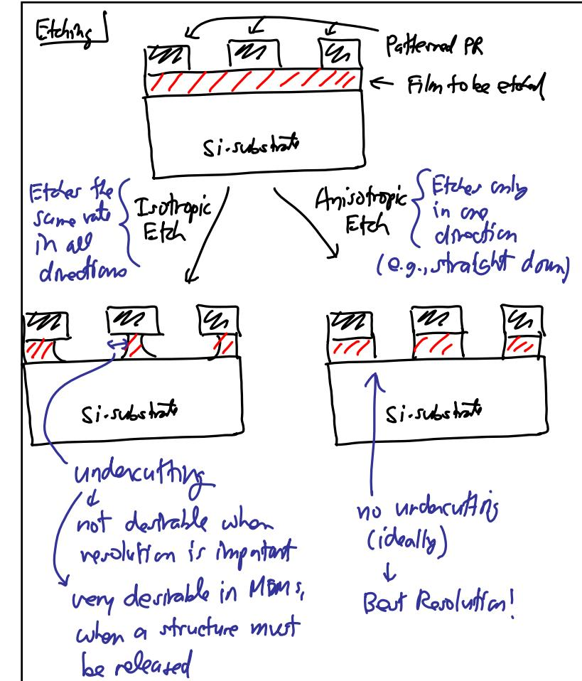
Example of Isotropic Etchants:
