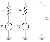
$$V_{\text{out}} = V_1 \left( \frac{R_2}{R_1 + R_2} \right) + V_2 \left( \frac{R_1}{R_1 + R_2} \right)$$
