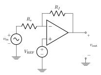
$$v_{\rm out} = v_{\rm in} \left( -\frac{R_f}{R_s} \right) + V_{\rm REF} \left( \frac{R_f}{R_s} + 1 \right)$$
