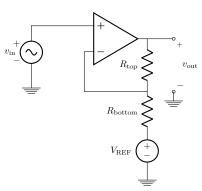
$$v_{\text{out}} = v_{\text{in}} \left( 1 + \frac{R_{\text{top}}}{R_{\text{bottom}}} \right) - V_{\text{REF}} \left( \frac{R_{\text{top}}}{R_{\text{bottom}}} \right)$$
