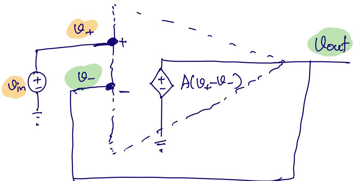
$$V_- = V_{out} \quad ; \quad V_{out} = A(V_+ - V_-)$$
