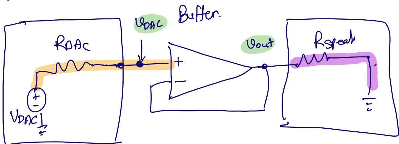
$$V_{out} = V_{DAC} !$$
