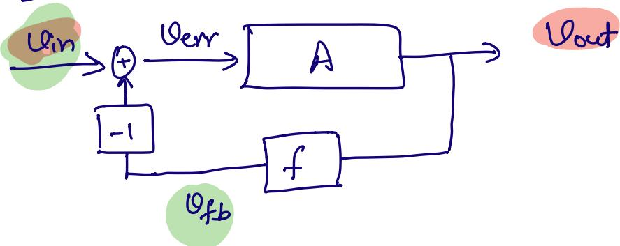
$$V_{in} - V_{fb} = V_{err} \quad ①$$
