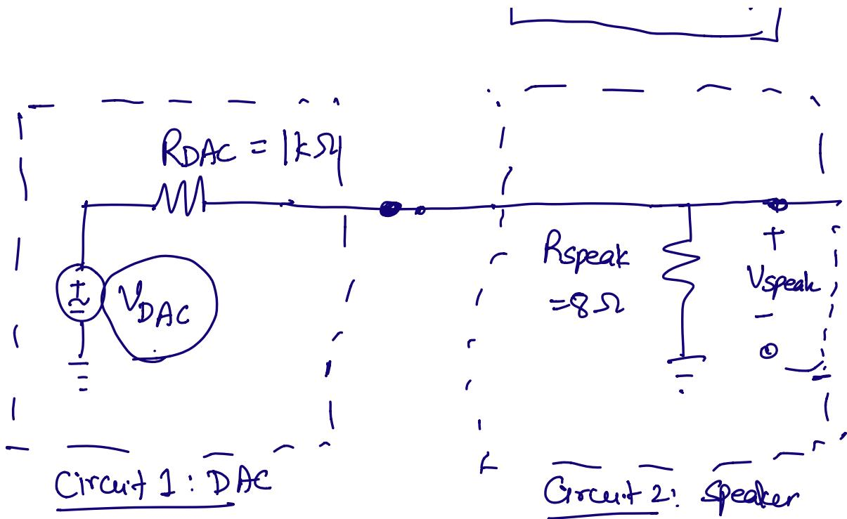
$$V_{speaker} = \frac{R_{speaker}}{R_{speaker} + R_{DAC}} \cdot V_{DAC}$$
