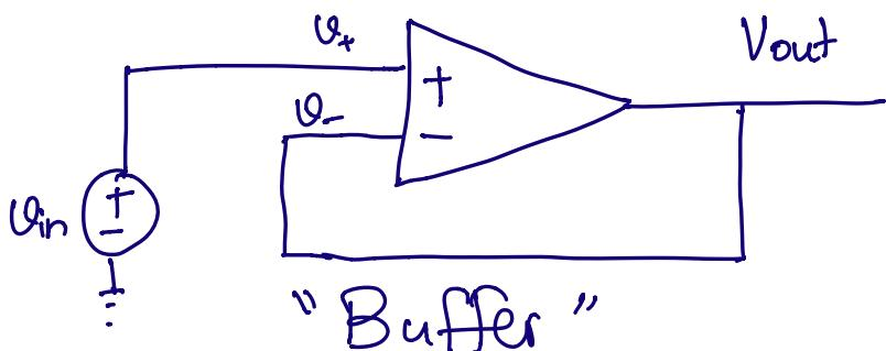
$$V_{out} = A(V_+ - V_-)$$
