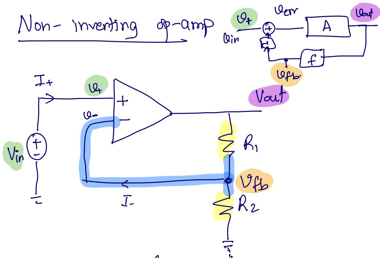
$$V_{fb} = V_{out} \cdot \left( \frac{R_2}{R_1 + R_2} \right)$$
