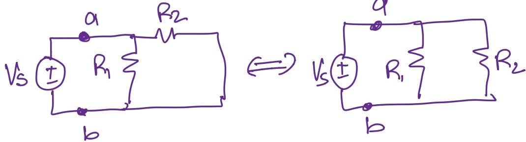
Superposition : Power of the linearity of circuits
