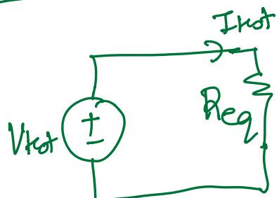
$$\bullet V_{\text{tot}} = I_{\text{tot}} \cdot R_{\text{eq}}$$
