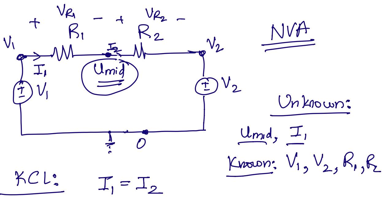
Element eqns:  $V_{R_1} = I_1 R_1$ ,  $V_{R_2} = I_2 R_2$
