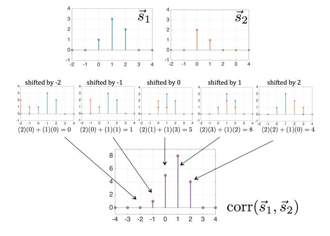
Eventually, the two signals no longer overlap (for example, when  $\vec{s}_2$  is shifted by -2 units). When the signals don't overlap, the inner product will be 0, since every non-zero element will be multiplied by zero. At this point we don't need to calculate more of the cross correlation. If we write all of the non-zero values in a vector, we get the following in this example:
