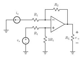
**Solution:** Using KCL at the  $v_-$  node we find that  $i_s = \frac{v_0 - v_-}{R_2}$  because, by the golden rules, no current flows into the opamp. Using the golden rules again we know that  $v_- = v_+$ . The voltage at  $v_+ = \frac{3R_1}{R_1 + 3R_1}V_s = \frac{3}{4}V_s$  which is the result of a voltage divider. Putting it all together we get:
