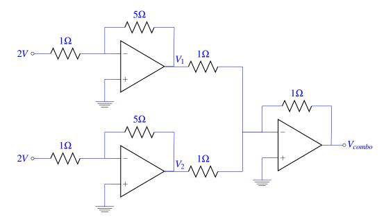
Using the result of part a),  $V_1 = -10V$  and  $V_2 = -10V$ . (Note that this would be true irrespective of what was connected to the outputs of the first two opamps. Think about why!) Now, let's look at the third opamp cascaded in the circuit. Now, using the result of part b), we'll get
