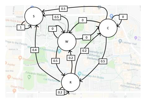
Figure 8.2: New DeliveryBot state transition diagram.
