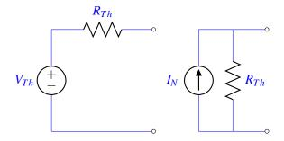
where  $R_{Th} = \frac{V_{oc}}{I_{sc}}$ . Plugging in a resistor *R* at the appropriate location, you end up with a voltage or current divider for Thevenin and Norton equivalent circuits, respectively. For completeness, we'll solve for both:
