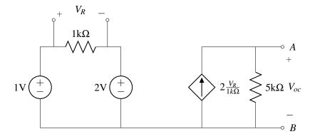
(a) Find the open-circuit voltage  $V_{oc}$  between nodes A and B.
