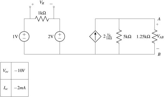
**Solutions:** For now, we'll work symbolically with  $V_{oc}$  and  $I_{sc}$ . With  $V_{oc}$  and  $I_{sc}$ , you can find the Thevenin and Norton equivalents of the circuit:
