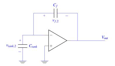
(e) (3 points) Find expressions for charge across each capacitor when  $s_2$  is on and  $s_1$  is off. **Solution:** Since the voltage on the positive terminal of this op amp in negative feedback is zero, the voltage on the negative terminal must also be zero. The charge across  $C_{tank}$  is given by:
