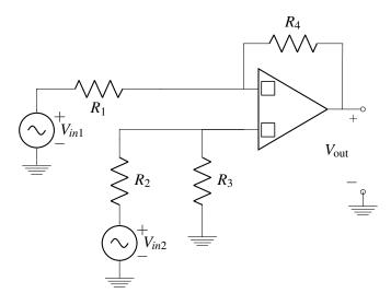
i. Label the '+' and '-' terminals of the op amp above so that it is in negative feedback. **Solution:**
