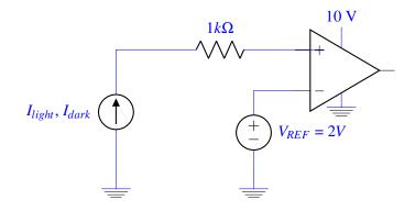
(b) (4 points) You realize that the light sensor can only provide a maximum of  $P_{max} = 40mW$  of power. Does this affect your design from part (a)? If so, how should it change? If not, why does it not affect it?
