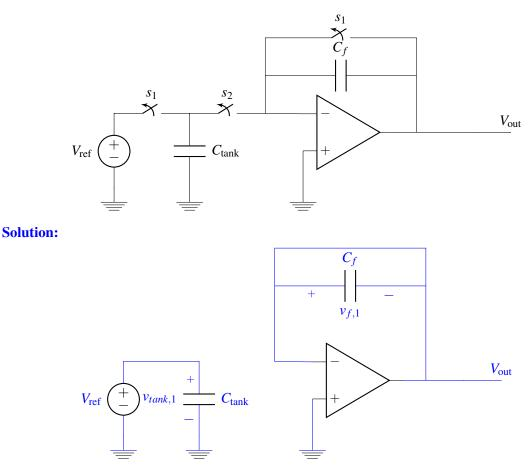
(c) (3 points) Find expressions for charge across each capacitor when  $s_1$  is on and  $s_2$  is off. Solution: The charge across  $C_{tank}$  is:
