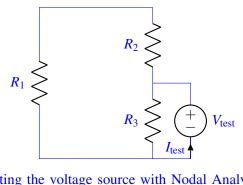
And calculate the current exiting the voltage source with Nodal Analysis or Resistor Equivalences. This solution uses resistive equivalences.  $R_{eq}$  as seen from the voltage source is
