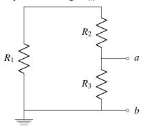
**Solution:** Start by finding  $V_{oc}$ , which is the voltage dropped across  $R_3$ . Since there are no sources in this circuit, the voltage across  $R_3$ ,  $V_{R_3} = 0$  and therefore  $V_{th} = 0$ . To find  $R_{th}$ , first null all independent sources (there are none). Then apply a test voltage to the terminals like so:
