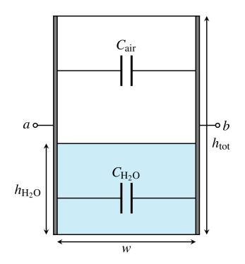
(a) (5 points) Derive an expression for the total capacitance,  $C_{\text{tank}}$ , between terminals *a* and *b* as a function of  $h_{\text{tot}}$ , *w*,  $h_{\text{H}_2\text{O}}$ , and  $\varepsilon$ .
