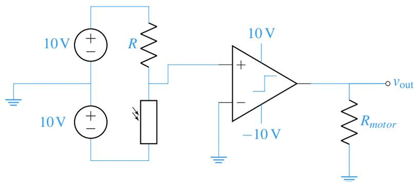
Since we have grounded the negative input terminal (and there is no feedback in the circuit), we realize the comparator rails high (positive  $v_{out} = +10$ V when the input to the positive op-amp terminal has positive voltage).
