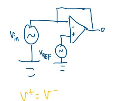
Chi would only work if  $V_{in} = V_{REF}$ , but it would not achieve the desired functionality of scaling  $V_{out} = S \cdot V_{in}$
