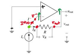
Calculate  $\frac{v_{out}}{v_{out}}$  as a function of  $\frac{I_s}{I_s}$  and R.
