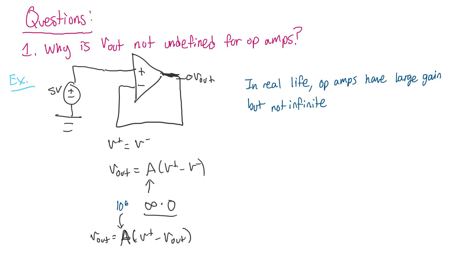
$$V_{ovt} = 10^{6} (5v - V_{ovt})$$
