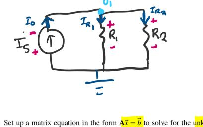
(e) Set up a matrix equation in the form  $A\vec{x} = \vec{b}$  to solve for the unknown node potentials and currents. What are the dimensions of the matrix A? Hint: you don't need to fill out the elements of A or  $\vec{b}$  in this part of the question.
