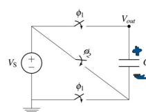
(a) In the circuit above switches  $\phi_1$  are initially closed and switch  $\phi_2$  is initially open. Calculate the value of the output voltage,  $V_{out}$  with respect to ground, and the amount of charge stored on capacitor, C, at
