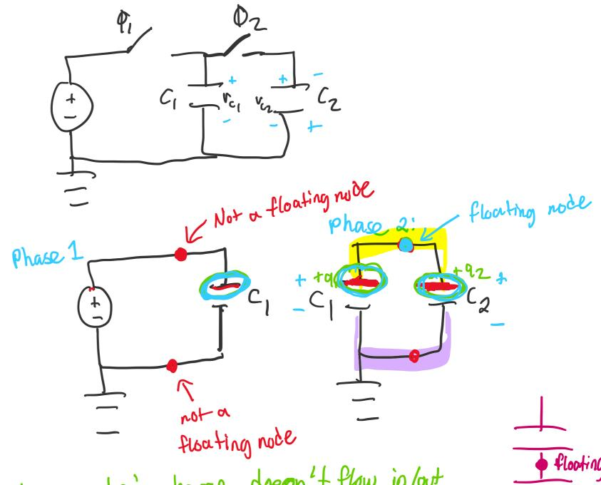
Floating node: charge doesn't flow in lout of the node
