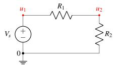
**Step 3:** Label the current through every element in the circuit " $i_n$ " so that every element has a current label. The direction of the arrow indicates which direction of current flow you are considering to be positive. At this stage of the algorithm, you can pick the direction of all the current arrows *arbitrarily*. As long as you are consistent with this choice and follow the rules described in the rest of this algorithm, the math will work out correctly.
