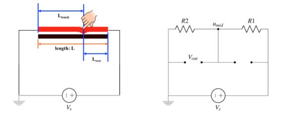
So why have the bottom plate at all? It lets us take the measurement for  $V_{out}$  using connection points on the edge of the plate instead of having to put a probe or wire at the actual touch point every time! As we have shown, in the case of an ideal bottom plate this does not affect the measurement result itself.
