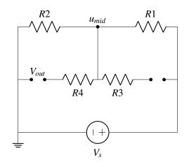
There are now more nodes in the circuit. We now have two options; we can either go back and perform nodal analysis with this new expanded circuit, or we can try and build off previous understanding to see if we can discern how the addition of resistors  $R_3$  and  $R_4$  affect circuit behavior.
