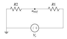
To understand what the bottom plate is doing, we will first assume it is a perfect conductor ( $\rho = 0$ ), so the circuit will look as follows. Notice again that a voltage source is connected to the terminating edges of the plates:
