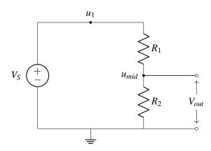
$$V_{out} = \frac{R_2}{R_1 + R_2} \times V_s. \tag{1}$$
