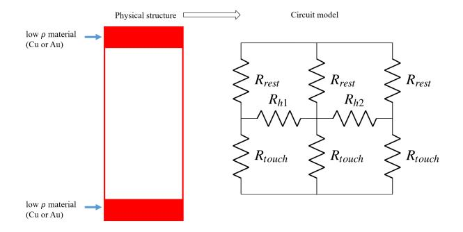
As we did with the 1D touchscreen, we connect a voltage supply  $V_s$  to the top and bottom ends of the top red plate:
