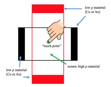
The top and bottom ends of the top red plate as well as the left and right ends of the bottom black plate are made of materials that have very low resistivities  $\rho$ , we can treat them as ideal wires ( $\rho = 0$ ). The materials of the transparent screen that we touch in the middle have much higher resistivity.
