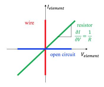
From the I-V plots, although a resistor, a wire and an open circuit can behave quite differently, their behaviors are exactly the same at (0, 0). This means that at (0, 0), these three circuit elements can be replaced by one another and the same behavior (I = 0, V = 0) is still expected.
