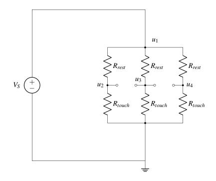
After replacing horizontal resistors with open circuit, we can use a voltmeter and measure  $u_3$ . Once again, using the voltage divider equation, we get:
