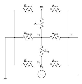
Once again, we see that this is very similar to the "interesting circuit" and we can replace  $R_{v1}$  and  $R_{v2}$  with open circuits. Then we perform the same analysis as for top red plate, and we can derive  $u_3$ , which is:
