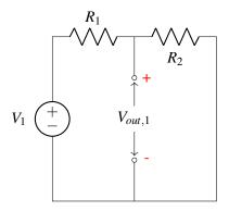
We can recognize this as a voltage divider circuit, and therefore we know that  $V_{out,1} = \frac{R_2}{R_1 + R_2} V_1$ . Next we compute the output voltage due to  $V_2$  and hence source  $V_1$  will be replaced with a wire.
