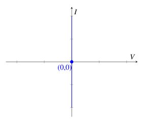
What does this mean? This means that it allows any current to go through, however the voltage drop always remains zero. This is exactly what a wire element (sometimes called a short circuit) does. Now let's look at why we replace current sources with open circuits. If we plot the I-V graph of a current source  $I_S$ , we get the following:
