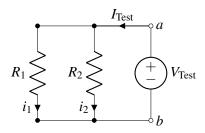
To analyze this circuit, first we notice that the voltage drop over each resistor is equal to  $V_{\text{Test}}$ . This is because the voltage drop between node a and b is  $V_{Test}$ , and each resistor is connected to node a on one side and node b on the other.
