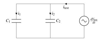
$$i_1 = C_1 \frac{dV_{test}}{dt}$$
