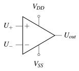
An op-amp has two input terminals marked (+) and (-) with potentials  $U_+$  and  $U_-$ , two power supply terminals called  $V_{DD}$  and  $V_{SS}$ , and one output terminal with potential  $U_{out}$ . The internal circuit design of an op-amp is beyond the scope of this course (if you are curious, you can search for schematics online), but we can model the op-amp with the following circuit:
