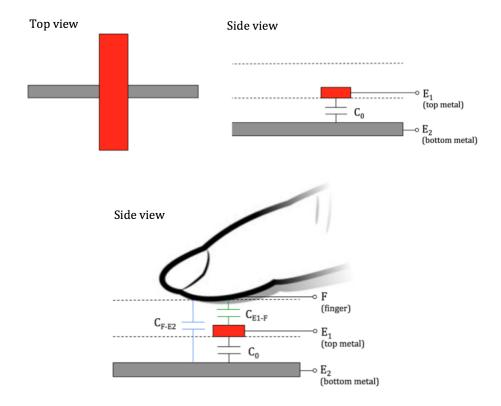
When the finger touches the top insulator, two new capacitors are formed between the finger and each of the two electrodes.  $C_{\text{F-E2}}$  is the capacitance between our finger (F) and electrode E2, and  $C_{\text{E1-F}}$  is the capacitance between our finger (F) and electrode E1. Now, we can draw the equivalent circuit model corresponding to the pixel we're looking at. Note that the nodes are labeled with the electrode or finger that the node represents.
