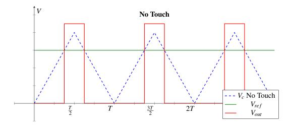
Every period of the current source cycle, we can measure if there is a finger touching this pixel. Later in this course, we will learn how to build a periodic current source like the one needed in this design — after that you will be ready to completely build your own capacitive touchscreen!
