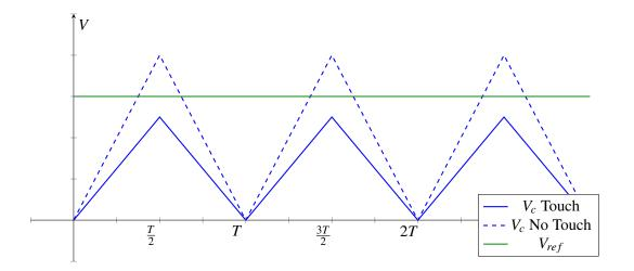
When there is a finger present,  $V_c$  is always less than  $V_{ref}$  so the output voltage is 0:
