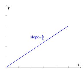
where t is the time passed since we started charging the capacitor. If we measure the voltage at a known time t, we can solve for the capacitance. However, as time continues to pass, the voltage across the capacitor (and also the charge stored on the capacitor) will grow to infinity. It is very challenging to build an ideal current source that works over this large range of voltages, so our model quickly becomes unrealistic.
