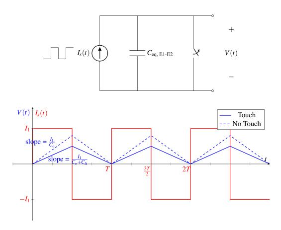
When there is no finger present, the slope of the rising edge of V(t) is  $\frac{I_1}{C_o}$ . When there is a finger pressing, the slope is smaller:  $\frac{I_1}{C_o + C\Delta}$ . This results in a smaller peak voltage when there is a finger press.
