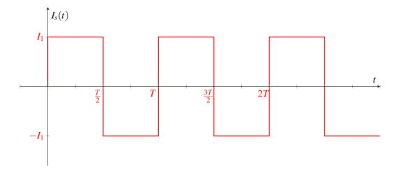
What does the voltage V look like with this current source? Let's assume that the capacitor is initially uncharged (ie. Q = 0). Since Q = CV, this means that at time t = 0 the voltage V = 0. (We will revisit this assumption later.)
