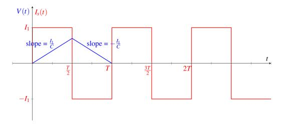
To determine the full behavior of V(t), we could continue to apply equation 4 for each period of constant current. However, we notice that at t = T, the voltage and current are the same as they were at t = 0. Since the current source is periodic (repeats every T), the voltage pattern will also repeat.
