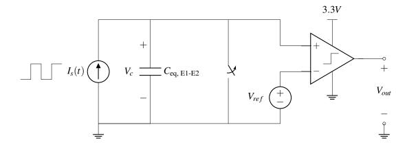
First, note that the voltage over the capacitor  $V_c$  is equal to the voltage at the positive terminal of the comparator  $(U_+ = V_c)$ . The negative terminal of the comparator is connected to  $V_{ref}$  so  $U_- = V_{ref}$ . Using the equations for a comparator, we can write
