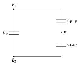
We can further simplify the circuit by replacing the series combination of  $C_{\text{E1-F}}$  and  $C_{\text{F-E2}}$  by some capacitance  $C_{\Delta}$ . When the finger is present,  $C_{\text{E1-F}}$  and  $C_{\text{F-E2}}$  have positive capacitance, so we know  $C_{\Delta}$  has some capacitance greater than zero.
