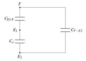
Our touchscreen can only measure things that are between electrodes  $E_1$  and  $E_2$  as it is impractical to physically connect a measuring device to our finger. So, we redraw our circuit as follows:
