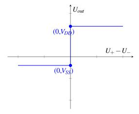
Since A is very large, there is a very sharp transition in the center of the plot. Therefore, when  $U_+ < U_-$  (or equivalently, when  $U_+ - U_- < 0$ ), then  $U_{out}$  equals  $V_{SS}$ . Similarly, when  $U_+ > U_-$ , then  $U_{out}$  equals  $V_{DD}$ . In this case, the op-amp is acting as a comparator since it indicates which voltage  $(U_+ \text{ or } U_-)$  is larger, even if the difference between them is very small.
