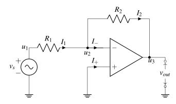
Let's assume that this circuit is in negative feedback so that we can use golden rule #2, after analyzing the circuit we will show how to check if a circuit is indeed in negative feedback.
