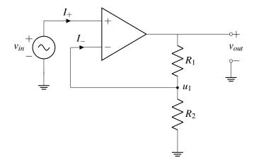
For the non-inverting amplifier circuit, we have
