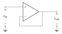
To analyze this circuit, we first notice that  $u_+ = v_{in}$  and  $u_- = v_{out}$ . We apply the second golden rule,  $u_+ = u_-$ , which tells us
