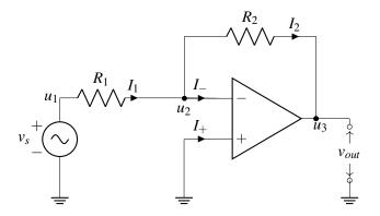
For the inverting amplifier circuit, we have
