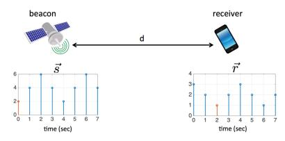
Our goal is to determine this time delay,  $\tau$ . Then we can use the velocity of radio waves (or light, or sound), v, to determine the distance:  $d = v\tau$ .
