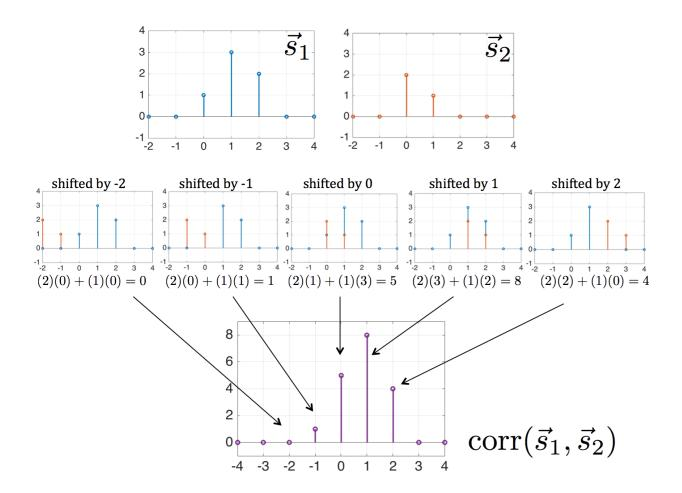
Eventually, the two signals no longer overlap (for example, when  $\vec{s}_2$  is shifted by -2 units). When the signals don't overlap, the inner product will be 0, since every non-zero element will be multiplied by zero. At this point we don't need to calculate more of the cross correlation. If we write all of the non-zero values in a vector, we get the following in this example:
