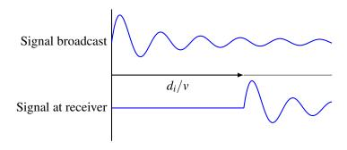
Notice that the received signal is delayed by some amount, due to its travel time. As we discussed earlier, letting  $d_i$  be the distance between the receiver and the beacon, this delay will equal  $d_i/v$ .
