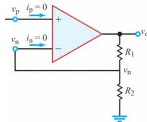
$$v_o = \frac{R_1 + R_2}{R_2} v_s$$
