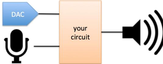
Let's assume that the microphone can be modeled as a voltage source with min/max values of 0 V and 1 V (relative to the DAC's ground) and a  $10\text{k}\Omega$  source resistance. However, because the materials in the headphones attenuate some of the external sound, the loudest signals picked up by the microphone should correspond to a voltage range of only  $-125\text{ mV}$  to  $+125\text{ mV}$  driven onto the speaker.
