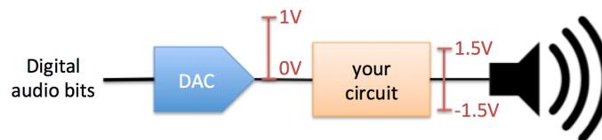
You are provided two voltage sources with values  $-1.5\text{ V}$  and  $1.5\text{ V}$ , an op-amp, and any resistors you would like. Design a circuit that could drive the speaker while meeting the specifications above. Draw a block diagram for the circuit you design before you actually determine the components necessary.
