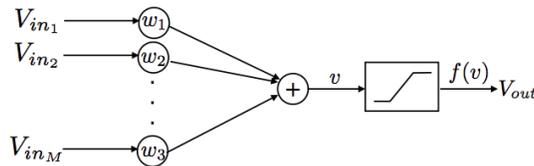
Input signals  $v_{in_i}$  are voltages from other neurons, which are multiplied by a constant weight  $w_i$  in each synapse and summed in the neuron. Each neuron also contains a nonlinear function (called a sigmoid) which is defined as
