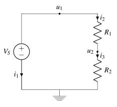
• Step 4: Add +/- labels on each non-wire element by following the passive sign convention.
