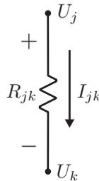
For resistor  $R_{jk}$  connecting nodes  $j$  (marked with + voltage polarity) and  $k$  (marked with - voltage polarity),
