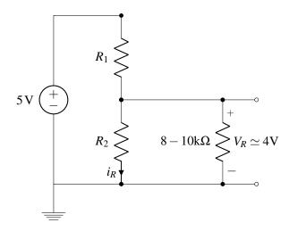
(e) For part (b), how much power does each element dissipate? Calculate the power using your Thévenin equivalent and using the original circuit. Are the values the same?
