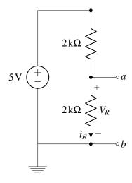
(b) What happens to the output voltage  $V_{ab}$  if we attach a load of  $8 \,\mathrm{k}\Omega$  to the output as depicted in the circuit below? Use your Thévenin equivalent from part (a).
