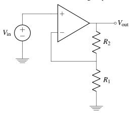
7. If we placed a buffer, which is an op-amp in negative feedback that has a gain of 1, between two subcircuits, would it be the same as connecting the subcircuits with a wire?
