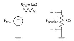
Using the voltage divider equation, we calculate that
