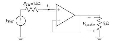
From the first golden rule, we know that  $i_+=0$ . This means there is no current through  $R_{TH}$ , and therefore no voltage drop across the resistor. In other words, the op-amp does not load the DAC since it has infinite internal resistance! Since there is no voltage drop over  $R_{TH}$ , we know that  $u_+=V_{DAC}$ . Combing this with our previous analysis of the buffer, we see that  $V_{DAC}=V_{speaker}$ , as desired.
