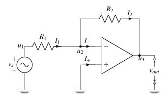
Let's assume that this circuit is in negative feedback so that we can use golden rule #2. After analyzing the circuit, we will describe how to check whether a circuit is in negative feedback.
