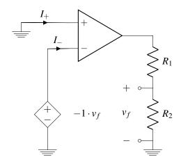
**Step 2**: If we increase  $v_{out}$ ,  $v_f$  increases which then decreases  $v_- = -1 \cdot v_f$ , which then increases  $v_{in} = u_+ - u_-$ , thus  $v_{out}$  increases. The circuit response to the increase in  $v_{out}$  is in the same direction as we "dinked"  $v_{out}$ . So this circuit is not in negative feedback.
