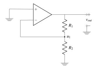
**Step 2**: If we increase  $v_{out}$ , we know  $u_1$  will increase because  $R_1$  and  $R_2$  form a voltage divider.  $u_1$  is connected to  $u_-$ , so  $u_-$  increases, therefore  $v_{in} = u_+ - u_-$  decreases, and thus  $v_{out} = Av_{in}$  decreases.
