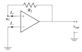
**Step 2**: If we increase  $v_{out}$ , we know  $u_1$  is going to increase because  $u_1 = v_{out}$ .  $u_1$  is connected to  $u_+$ , so  $u_+$  increases, therefore  $v_{in} = u_+ - u_-$  increases, and thus  $v_{out}$  increases. So the feedback from the circuit is in the same direction, and this circuit is not in negative feedback.
